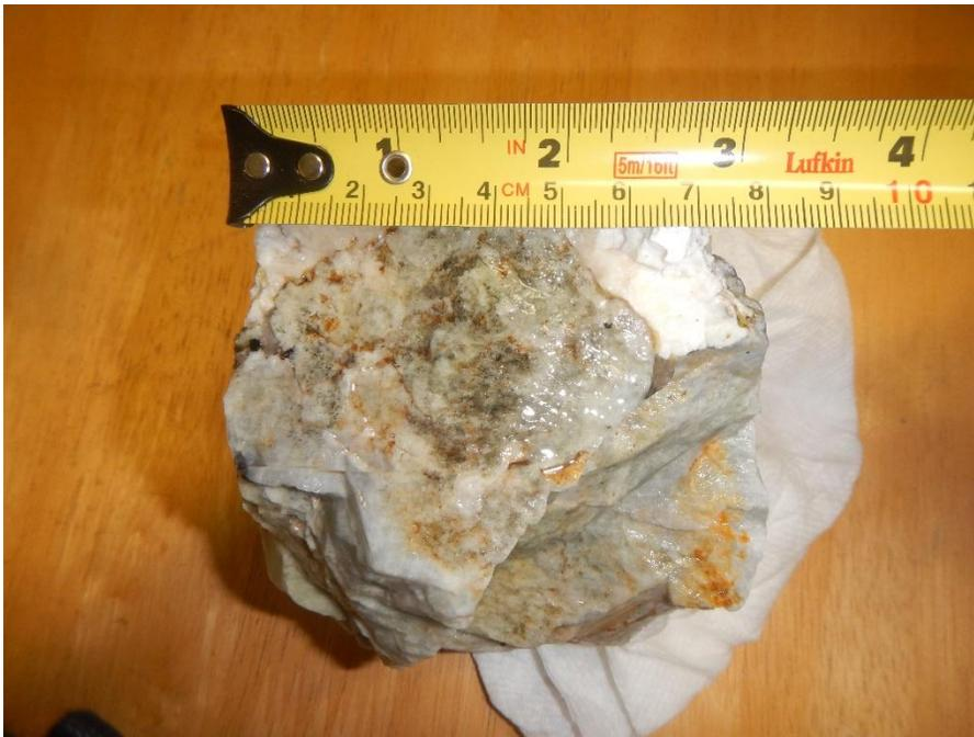
*Figure 2: Photo of pale green 6 cm diameter spodumene crystal from Dome 9, Case Lake..*
