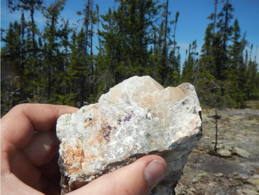
Figure 3: Photo of purple lepidolite (Li-mica) from 10 m wide dyke near the spodumene dyke on Dome 9, Case Lake.
